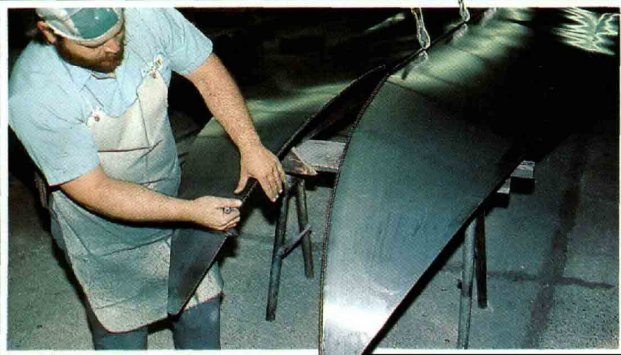
Below —At Lund, flanges are manually bent into the curved portions of the bottom panels with Vise-Crips, which serve to close the straight, machine-bent run of the centerline seam.
