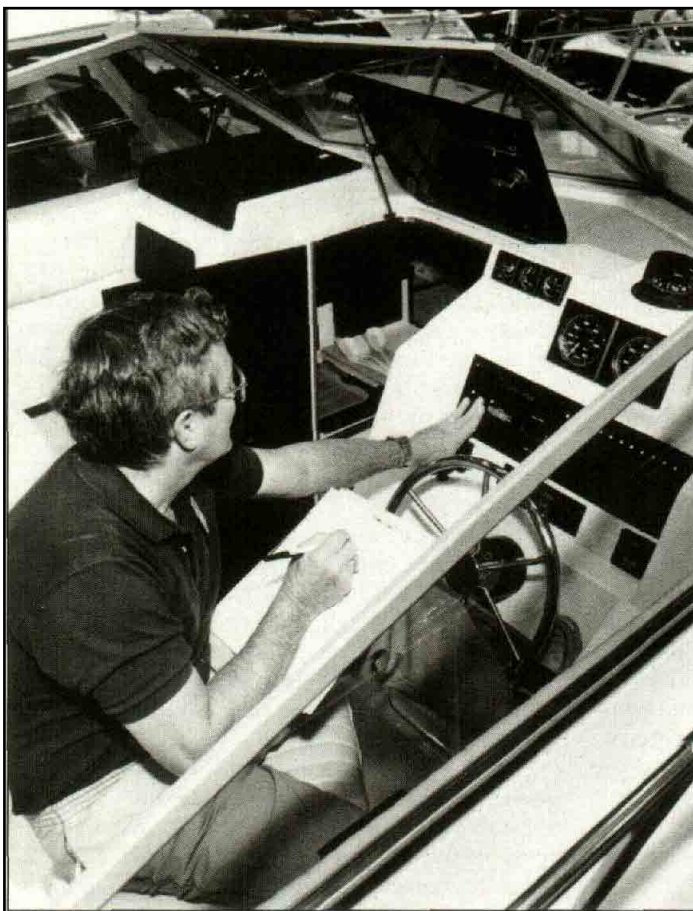
Among its other services, the National Marine Manufacturers Association (NMMA) offers a certification program. Here, one of the group's engineers inspects the dash of a new boat for compliance with government and industry construction standards.
