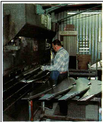
Below —At Lund, flanges are manually bent into the curved portions of the bottom panels with Vise-Crips, which serve to close the straight, machine-bent run of the centerline seam.
