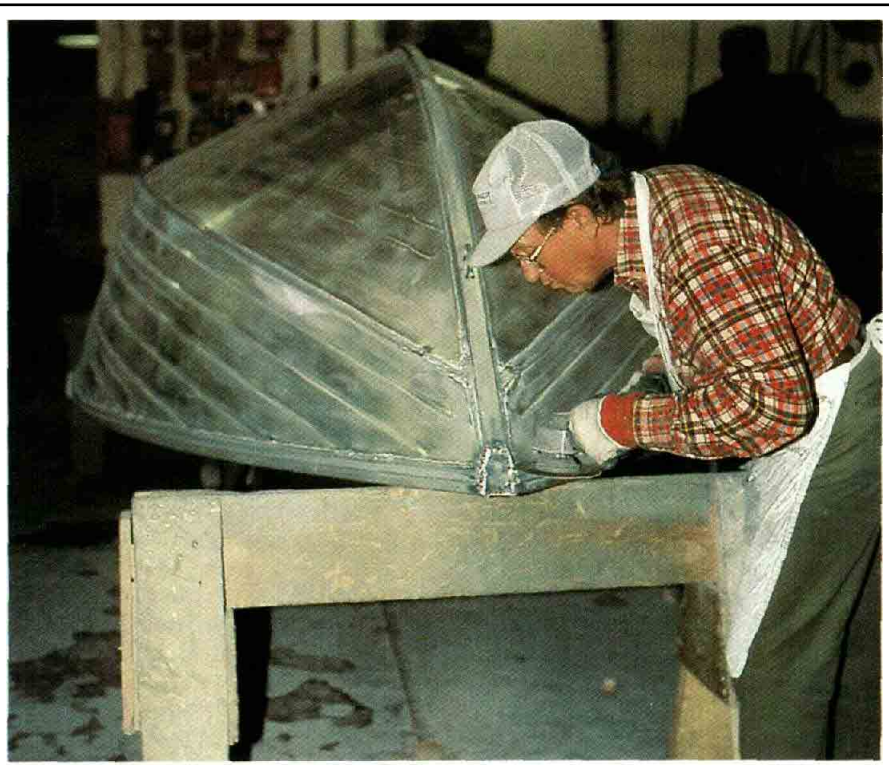
Below— A Crestliner employee grinds down a weld on the stem of a V-bottomed skiff. After this "rivet-free" boat is etched and painted, its seams will almost be invisible.
