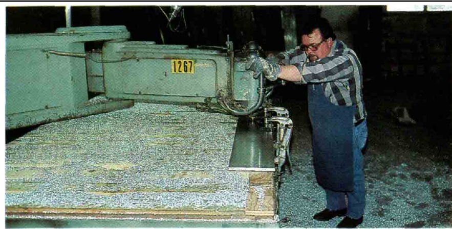
Above —A Lund employee manipulates a "broken arm" router as he cuts components out of aluminum stock.
