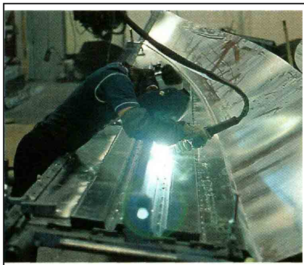
Left— Welding transverse and longitudinal hull stringers into place eliminates the need to bend flanges into these stiffeners to provide an anchor point for rivets. The torch, however, requires more finesse than the rivet gun.
