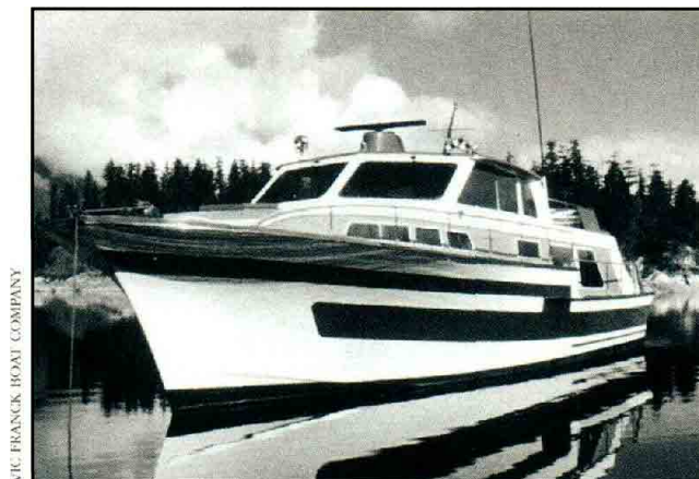
Launched in 1970, this is one of the first pleasure boats built with turbine engines. Two Pratt and Whitney JP-6 turbines give the 58-footer a 34-knot cruising speed.
