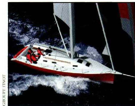
The South 35 is Finot's newest production racer/cruiser. Construction is carbon pre-preg; the builder, Aerodyne Technology in South Africa. She measures 34.4' (10.5m) by 11.5' (3.52m). Groupe Finot's name for the rig is the "C. Wing."
