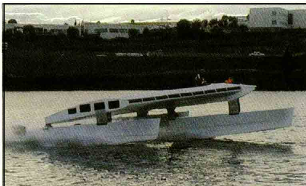
Next-generation Incat ferries may look like this scale-model being tested by company chairman Robert Clifford, who reports high speeds and good maneuverability from the unusual swept-wing design.
