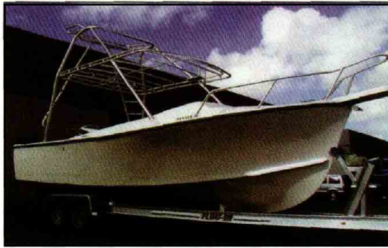
Florida builder Kick Dee KY/S commissioned to build a special edition of his stock 24-footer, designed and molded by Paul Morgan. The deluxe version of Dee's Marineteck commercial and sportfisherman is powered with twin Yanmar turbodiesels, and finished with plenty of teak and custom-made hardware.
