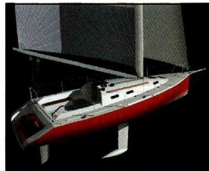
The South 35 is Finot's newest production racer/cruiser. Construction is carbon pre-preg; the builder, Aerodyne Technology in South Africa. She measures 34.4' (10.5m) by 11.5' (3.52m). Groupe Finot's name for the rig is the "C. Wing."
